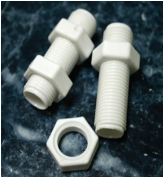
(FIG 4) Here you can see the bulkhead with a gasket flush against the stationary nut, forming a tight seal that will lock over the outside of the yeast collection vessel.
