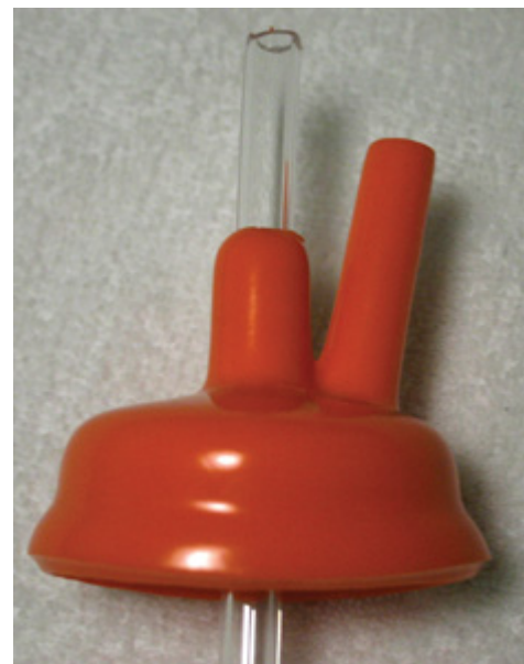
(FIG 9) Here is the carboy cap with a modified racking cane inserted. This will allow for hook up to the collection vessel.
