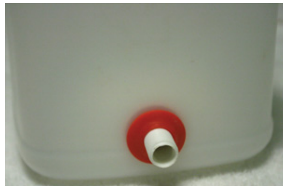
(FIG 6) The bottom bulkhead with the outer gasket seated for a snug fit.
