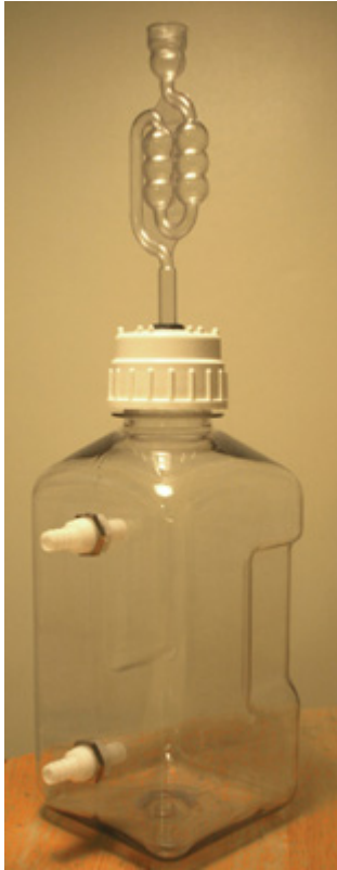
(FIG 10) An alternative collection vessel design, using a 2-liter Nalgene LEXAN square bottle.
