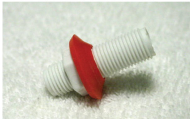
(FIG 4) Here you can see the bulkhead with a gasket flush against the stationary nut, forming a tight seal that will lock over the outside of the yeast collection vessel.
