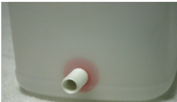
(FIG 5) Here is the bottom bulkhead inserted into the collection vessel that will help circulate the yeast.
