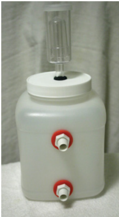
(FIG 9) Here is the carboy cap with a modified racking cane inserted. This will allow for hook up to the collection vessel.
