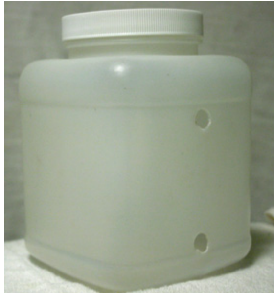
(FIG 2) The collection vessel now has two 1/2-inch holes drilled to accommodate the bulkhead fittings.
